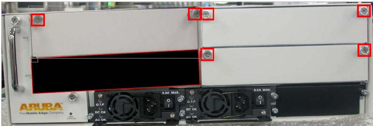
2. Remove the fan module, PSUs and blank PSU.
