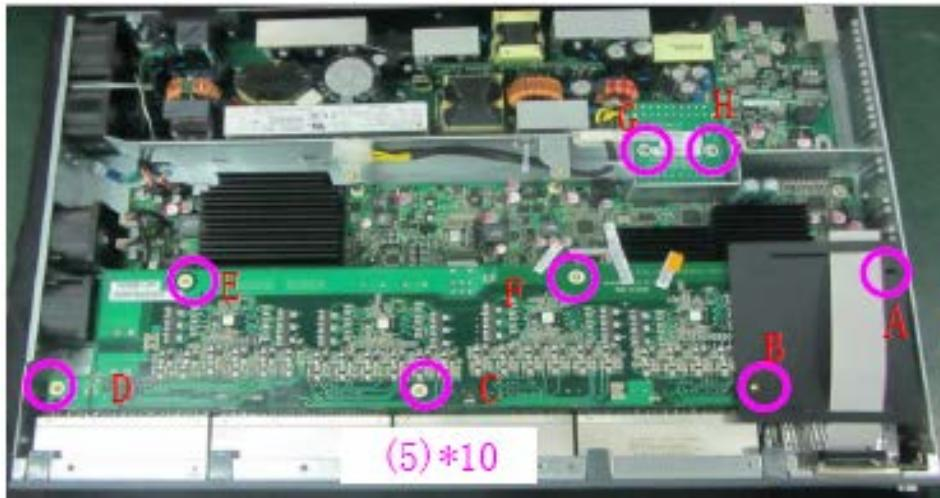
3. Remove the power supply unit and the console board.
