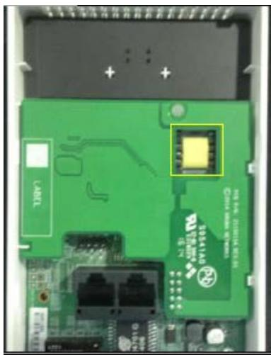
3. Remove the main board from the chassis.
