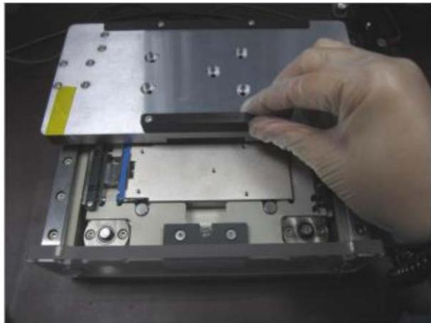
1. a) Place the module into the top screwing assembly fixture.
