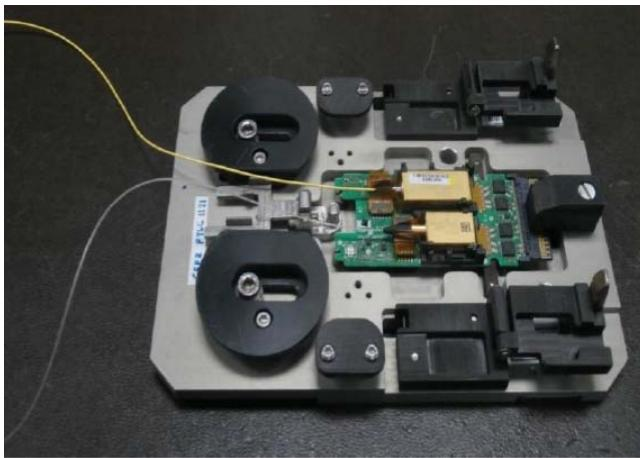
7. Place the PCBA into the carrier or in-process tray.
