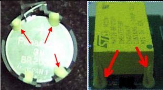
Figure 2 Clear the yellow adhesives by the tweezers.
