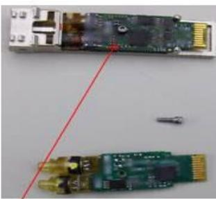
5. If present, remove screw holding PCA to housing
