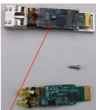
5. If present, remove screw holding PCA to housing
