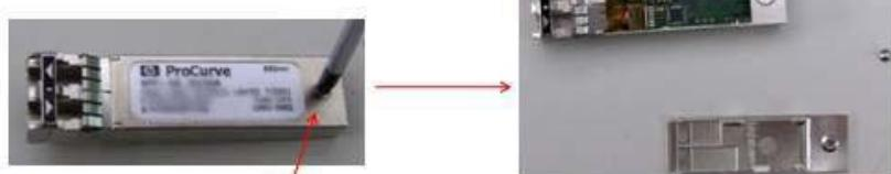
3. If screws are used to hold housing together, remove using correct screwdriver
