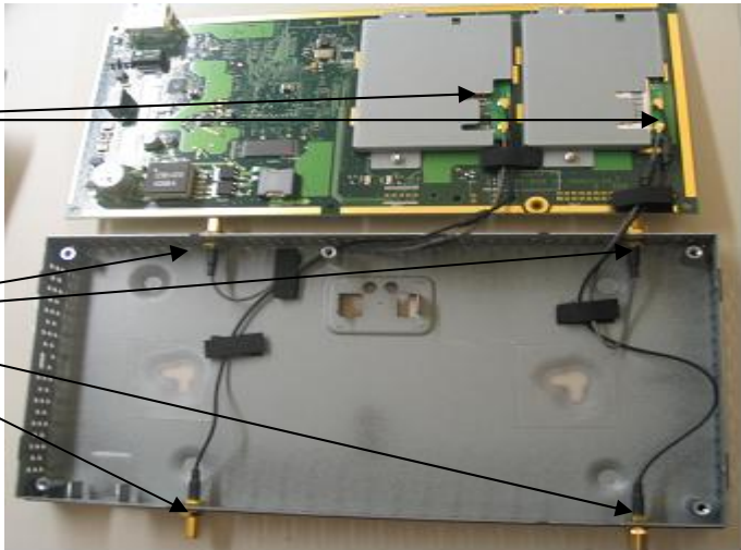
Fig. II – Open these screws to remove PCB from chassis and radio shields
